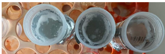
Appendix D. Degradation time of UCL-Ch-CTZ during the drug release assay after 24 hours
