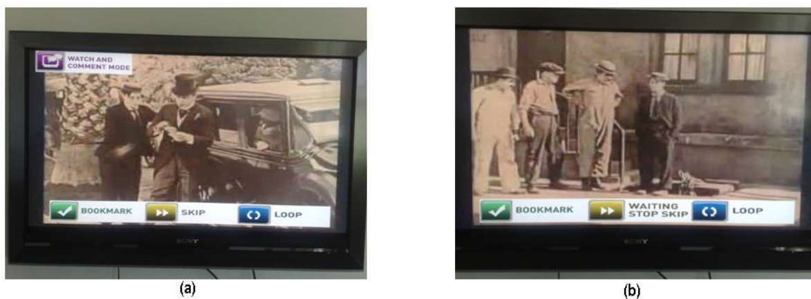
Figura 2.4: (a) Viewer has entered EDIT mode and presses the yellow triangle bottom associated with the start of a SKIP sequence. (b) The prototype replaces SKIP by WAITING STOP SKIP to indicate that the end of the skip sequence is expected
