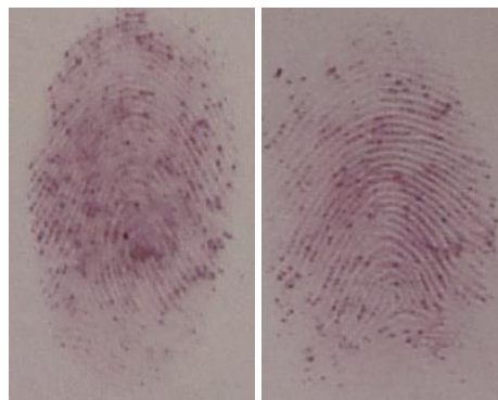
Figure 03: Obtained images for several deposition pattern times and temperatures between 85^\circ\text{C} \pm 0.5^\circ\text{C} e 145^\circ\text{C} \pm 0.5^\circ\text{C} , on cardboard samples.
