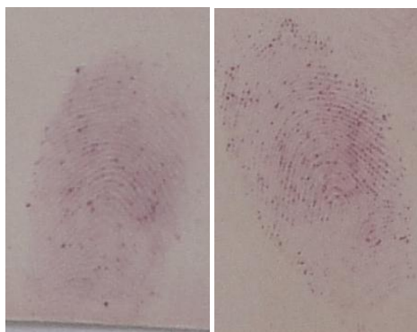
Figure 01: Obtained images for deposition pattern time of 3 s, subjected to a temperature of 85^\circ\text{C} \pm 0.5^\circ\text{C} , on cardboard samples.
