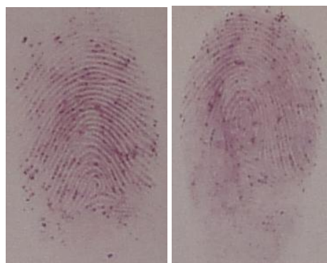
Figure 05: Obtained images for several deposition pattern times and temperatures between 85^\circ\text{C} \pm 0.5^\circ\text{C} e 145^\circ\text{C} \pm 0.5^\circ\text{C} , on cardboard samples.
