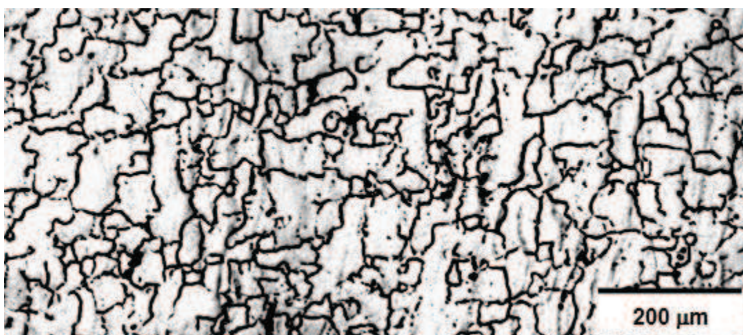
(f) T = 1200^{\circ}\text{C} , D = 17,75\mu\text{m} , \varepsilon = 4,0
