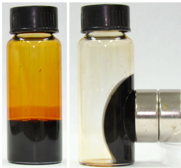
Figure 3.7. Photography of vials containing maghemite colloidal dispersion without the influence of magnetic field and under the influence of an external magnetic field. We can notice that there is no phase separation between the nanoparticles and the solvent. The entire dispersion is attracted by the magnetic field. This is a typical behavior of MR fluid.
