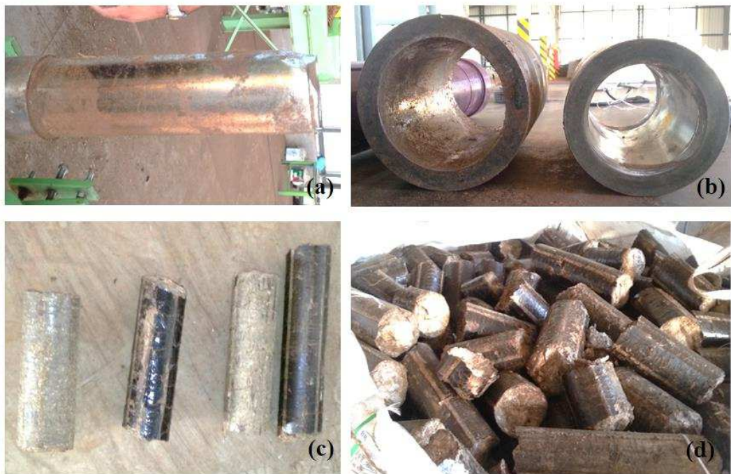
Figure 12 - (a) Frayed piston of a briquetting machine; (b) Cylindrical molds for briquetting machine; (c) Not uniform briquettes; (d) Briquettes of sugarcane trash.
