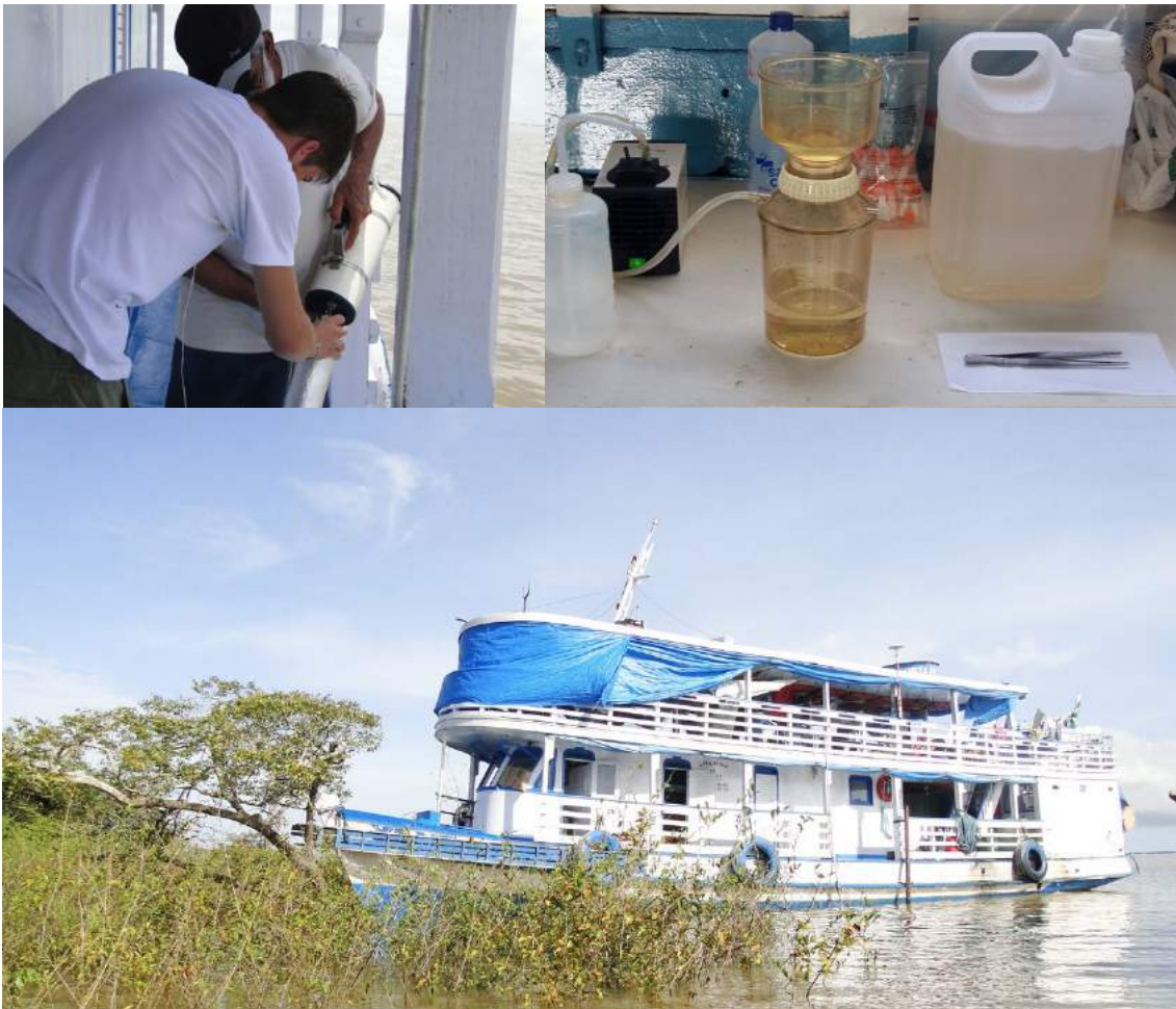
Supplementary figure I - 5: Sampling procedures (water collect with Van-Dorn bottle and filtration) and field workstation. Source: Leonardo Gomes.
