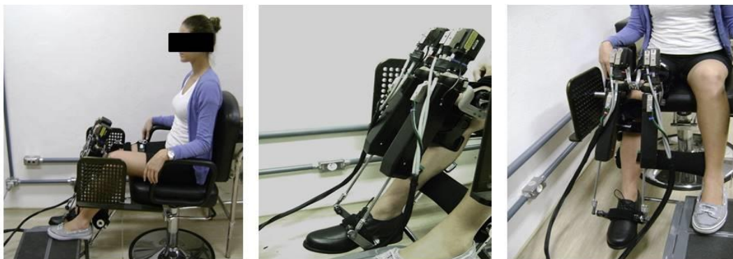
Figure 2: Image of patient positioned in the anklebot during the game task.
