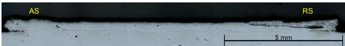
Figure 5.9 - Cross-sections extracted from the beginning of the coatings generated by 2-A configuration. The cross-sectional area is noticeably lower than the ones observed on samples extracted from the middle section of the coating, which is a product of a lower deposition efficiency during this stage of the process.
