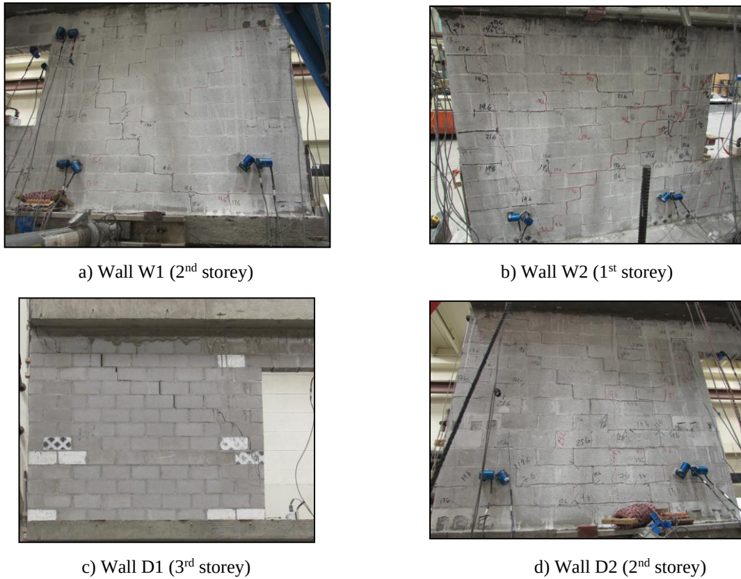
Figure 55: Damage mechanisms observed in experimental tests.
