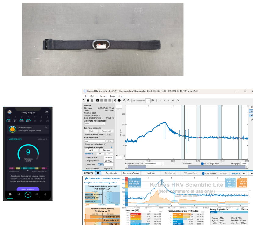
Figura 12. Transmissor cardíaco bluetooth - H10 Polar®, aplicativo Elite HRV: Wellness & Fitness® e software Kubios HRV®
