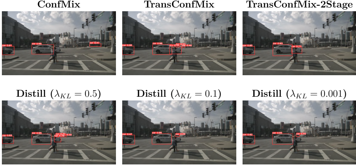
Figure 13 – Qualitative comparison of detection results for the DOLPHINS \rightarrow nuScenes scenario. Each panel shows representative predictions obtained with the evaluated adaptation methods on the same target-domain image
