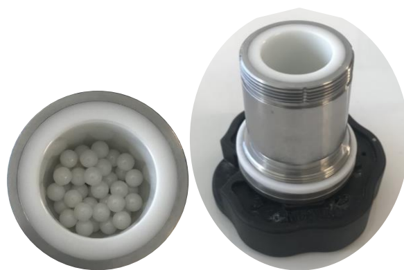
Figure III.2 – Grinding jar made of zirconium dioxide filled with 50 zirconium dioxide balls.
