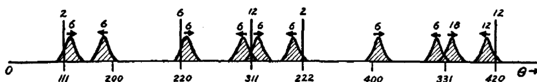
Figure 4.14: Representation of FCC peak displacement due to deformation faults [152].
